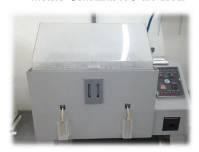
✓ Corrosive resistance is checked in salt spray camera according to Russian standard GOST 9.308.
